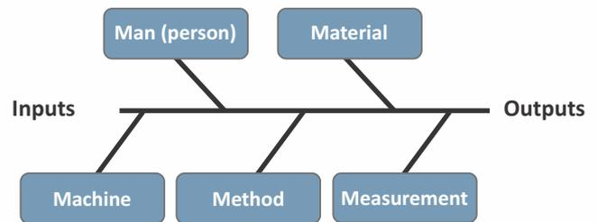
Figure 2: The Basic Fishbone Diagram
